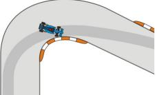
Notice that with both of these handling characteristics, it's what the car is doing, not what you're doing. In other words, oversteering is not when you've steered the car too much, and understeer is not when you've steered too little.
