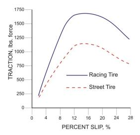
Driving a car at the limit is driving with the tires at their peak slip angle. If a tire generates its maximum traction with five degrees of slip, and you're driving with them at three degrees of slip, you're not driving at the limit. If you're driving with the tires at seven degrees of slip, you're driving beyond the limit.
